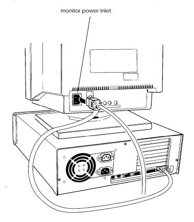
6. Plug the other end of the power cord into an appropriate grounded electrical outlet or, if the cord has the correct type of plug, into the power outlet on the back of the computer.
